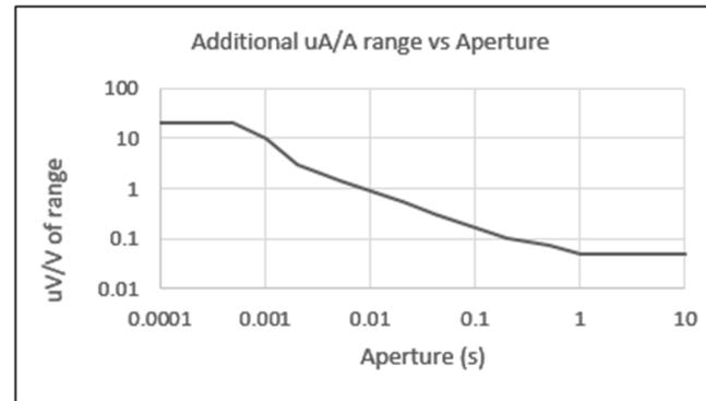
Aperture  $\geq 100 \mu\text{s}$ ; additional uncertainty with read rate
