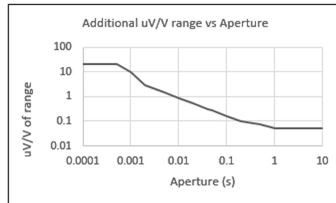
**Read Period Specification**Aperture  $\geq 100 \mu\text{s}$ ; additional uncertainty with read rate: (Period = aperture + delay between readings)
